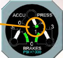
If not, recharge the accumulator using the YELLOW electric pump (SA aircraft), or the BLUE electric pump (LR aircraft).
