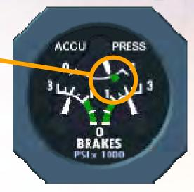
To ensure parking brake availability, in case emergency braking is required during pushback due to a broken towbar.
