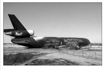
*The left side of the fuselage and the left wing received minimal damage by the impact and fire.* (Photo: U.S. National Transportation Safety Board)
